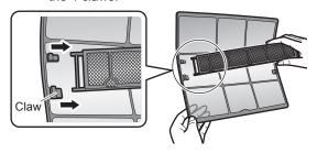
**2.** Clean or replace the titanium apatite photocatalytic airpurifying filter and the silver particle anti-bacterial filter (Ag-ion filter).
